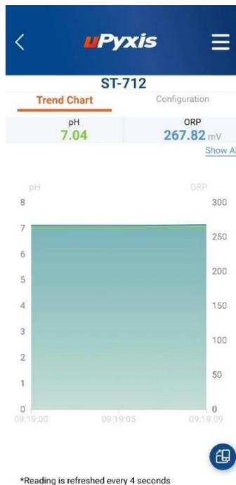
Tap **Configuration** on the top of the app page to launch the configuration page. Six functional tabs of each are available on this page: Information, Configuration, Calibration, 4-20mA Span, Diagnosis and User Guide.
