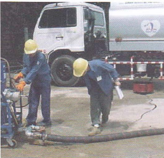
Because the life expectancy of the hose is limited, the user must be alert to signs of impending failure, particularly when the conditions of service include high working pressures and/or the conveyance or containment of hazardous materials.
